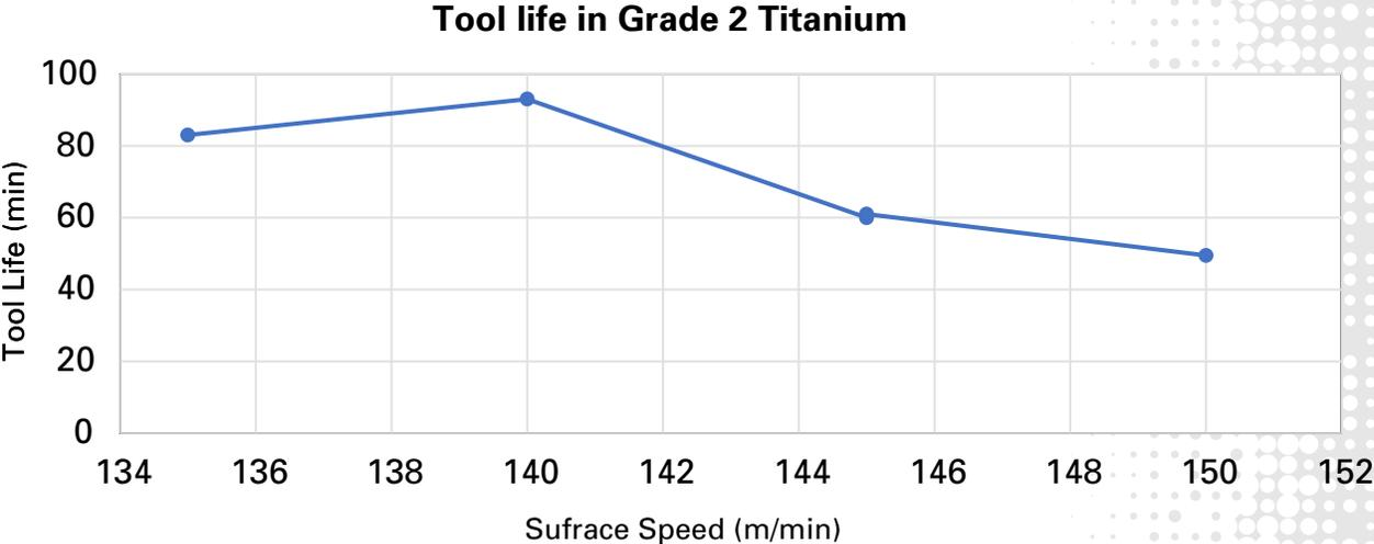
Figure 3. Tool life in Grade 2 titanium
