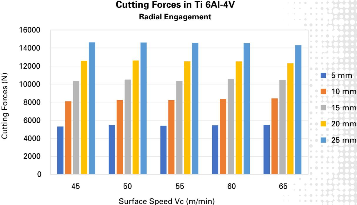
Figure 4. Cutting forces in Ti 6Al-4V
