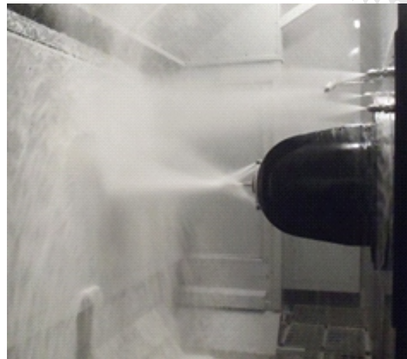
Figure 4. T4 machine high-flow coolant systems
