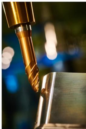
Then, the small radius tip of the tool can get into tight corners. Not only can manufacturers do more with a single tool, it results in continuous machined surfaces with significant reductions in blending issues. Barrel-shaped milling tools also come in multi-flute configurations. Add it all up, and the result is fewer tool passes with better surface quality, faster feed rates, less tool changes and a more productive cutting process.
