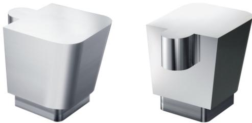
A final example looks at the finishing of a sloped surface in a mold cavity. Traditionally, on a 3-Axis machine, this surface would have been developed using a Z-Axis stepping technique and a ball nosed end mill. However, using a ball nosed end mill on a 5-Axis machine, the final, finished surface can be generated in a single machining pass. Obviously, this saves time, extends tool life, requires fewer tools and toolpaths and generates a better surface finish.
