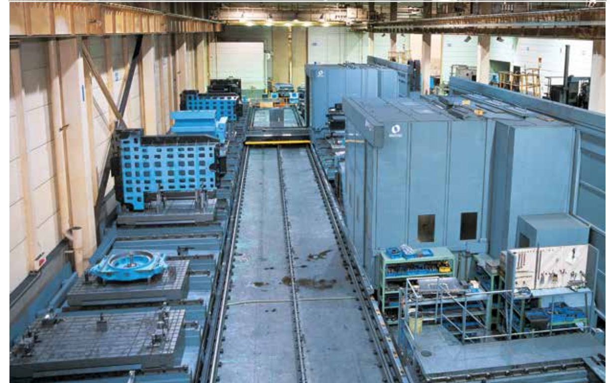
(Large Horizontal Machining Centers x 2) + (19 Pallets)
