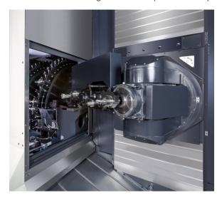
By increasing the spindle power from 120 kW to 130 kW in the updated models, maximum power can be achieved at 26,000 rpm rather than 33,000 rpm with the previous spindle. Cutting feed rates and acceleration rates have also been improved with cutting feed rates nearly doubling from 25.4 m/minute to 50 m/minute and acceleration rates reaching 1G. Together, these enhanced features dramatically improve processing speeds for all aluminum structural type components.
