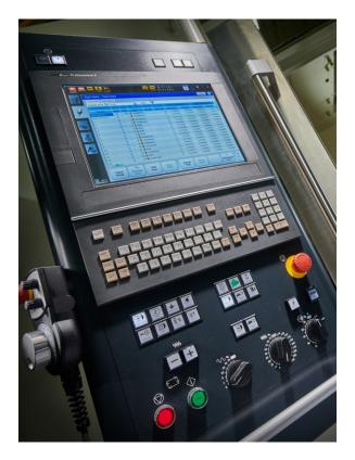
The Makino Pro6 High Performance Control provides the perfect blend of Microsoft Windows 7 OS graphical user interface (GUI), networking and storage capability with the proven stability of Fanuc hardware. It features a highly integrated, embedded control system capable of fast execution of commands, high reliability, flexibility, integration capability and ease of operation.
