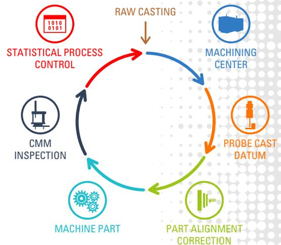
In a highly automated cell, some closed-loop providers have software with a graphics panel that displays CMM results and helps the operator monitor the machines. They are able to review robot speed control, cell sequencing, KPV reporting, feature correction and coolant monitoring. This information is valuable as it can quickly show that the closed-loop process is performing properly.
