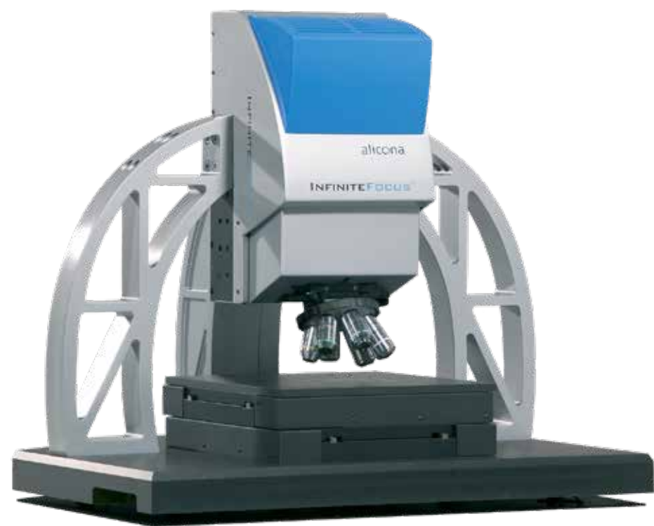
Alicona / IFM G4 Micro Coordinate Measurement System (Images courtesy of Alicona)
