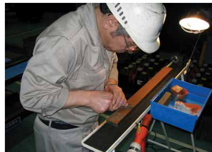
Hand scraping of guideway surface.
