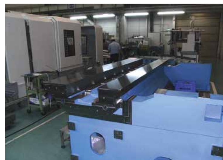
Precision ground and lapped guideway surfaces.
