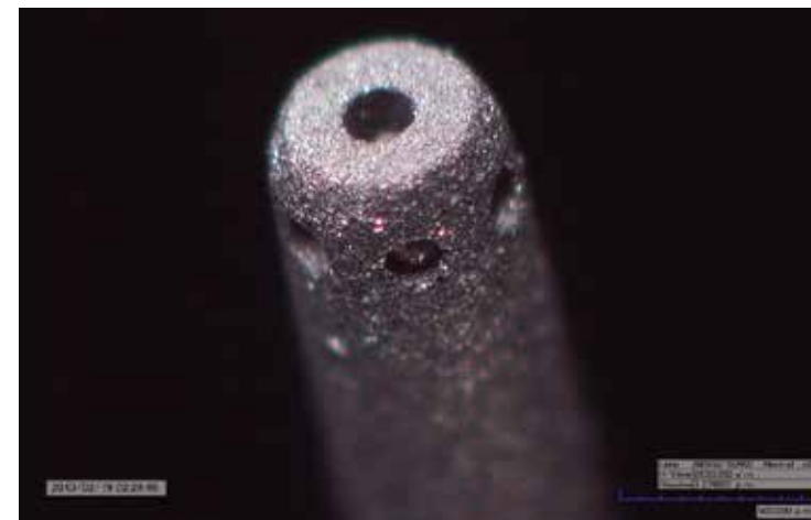
Image of \varnothing 120\mu\text{m} cross holes
