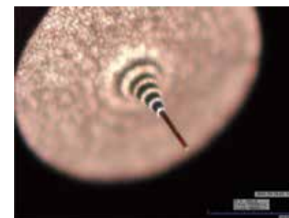
Dressed electrode: \varnothing 14\mu\text{m}
