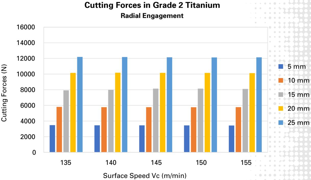
Figure 5. Cutting forces in Grade 2 titanium
