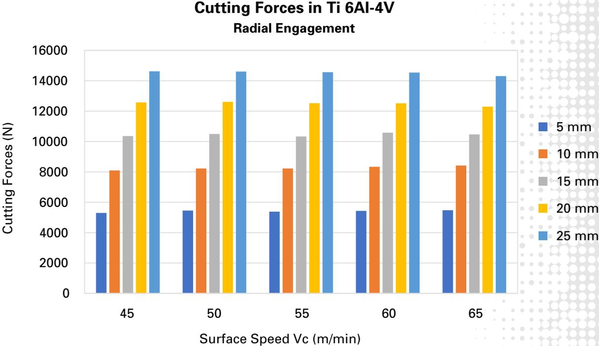
Figure 4. Cutting forces in Ti 6Al-4V
