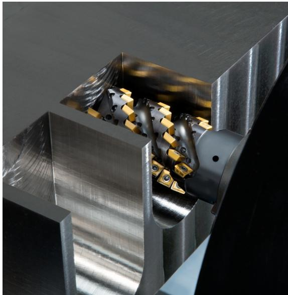
The conventional wisdom says that alloys other than Ti 6Al-4V require the surface speed to be reduced by 30-50%. (If you thought machining titanium was slow at 50 m/min (165 sfm), wait until you start machining at 25-35 m/min (82-115 sfm).
