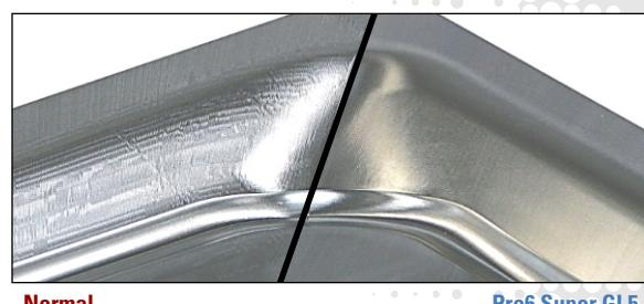
One of the ways SGI.5 achieves this superior finish is by maintaining a consistent velocity while cutting. Two machines, one Makino with SGI.5 and one competitor ran the same code on a complex surface. Sensors were used to measure velocity at each point during the program execution.
