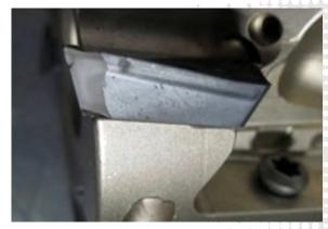
Figure 1. Tool wear observed on a high-performance machining center after 38 roughing passes in 4140 alloy steel. Replenish cost was \$60 for four new inserts.
