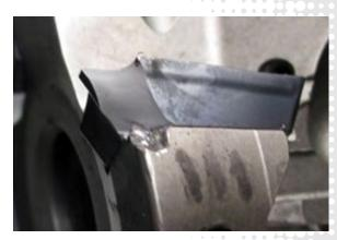
Figure 2. Tool wear observed on a conventional machining center after 28 roughing passes in 4140 alloy steel. Replenish cost was \$924 for four new inserts and a tool body replacement.
