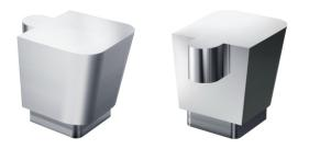
A final example looks at the finishing of a sloped surface in a mold cavity. Traditionally, on a 3-Axis machine, this surface would have been developed using a Z-Axis stepping technique and a ball nosed end mill. However, using a ball nosed end mill on a 5-Axis machine, the final, finished surface can be generated in a single machining pass. Obviously, this saves time, extends tool life, requires fewer tools and toolpaths and generates a better surface finish.
