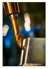
Then, the small radius tip of the tool can get into tight corners. Not only can manufacturers do more with a single tool, it results in continuous machined surfaces with significant reductions in blending issues. Barrel-shaped milling tools also come in multi-flute configurations. Add it all up, and the result is fewer tool passes with better surface quality, faster feed rates, less tool changes and a more productive cutting process.
