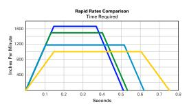
In the image above, the time required for a 10" move includes the profiles of four popular VMCs, all but one of which have similar published rapid rates. However, the top machine performed 30 percent faster than the slowest over just a 10-inch move. The longer the moves, and the more of them, the greater that difference becomes.
