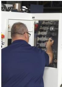
shorter distance to table for setup, overhead access to permit the use of a crane for heavy part or fixture loading, easier access to the tool changer for tool maintenance and exchange.
