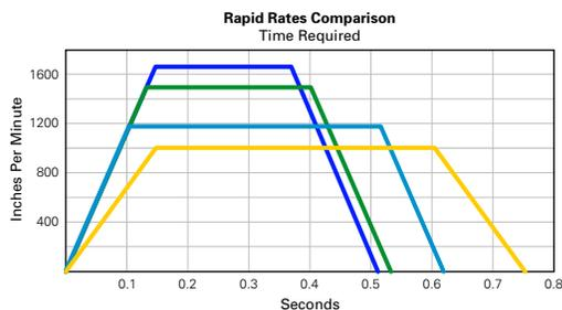
In the image above, the time required for a 10" move includes the profiles of four popular VMCs, all but one of which have similar published rapid rates. However, the top machine performed 30 percent faster than the slowest over just a 10-inch move. The longer the moves, and the more of them, the greater that difference becomes.
