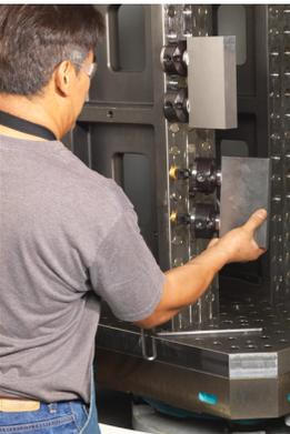
Standardize pallets and zero-point work-holding fixtures. This step is critical to enable your shop to run workpieces of different sizes in one cell.
